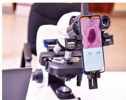
Adapter fixed on microscope holding the smart phone
